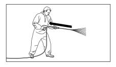
When using high pressure water for cleaning, make sure that there is a clearly noticeable recoil effect on the lance. Therefore ensure a firm footing (see chapter "Technical Data")
