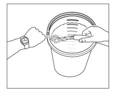
Lack of water occurs more often than you probably believe. The more powerful a high-cleaner is the greater is the danger that a lack of water occurs. If there is only an insufficient amount of water available, cavitation (water-gas mixture) arises inside the pump, which is normally noticed too late or even not at all. **The pump will be destroyed**. Please check the available quantity of water by filling a bucket with liter scale for one minute.
