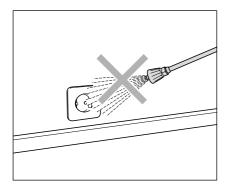
Never direct the water jet at power sockets or any other electrical installations!
