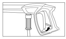
Apply the safety catch on the spray gun after each use in order to prevent unintentional spraying!
