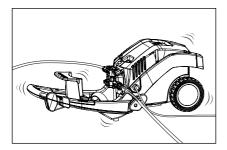
Having closed the trigger gun with safety catch, the HP cleaner must shut down. Failure to shut down may be caused by leakage in the pump, the Pressure Switch, the high pressure hose or the lance.
